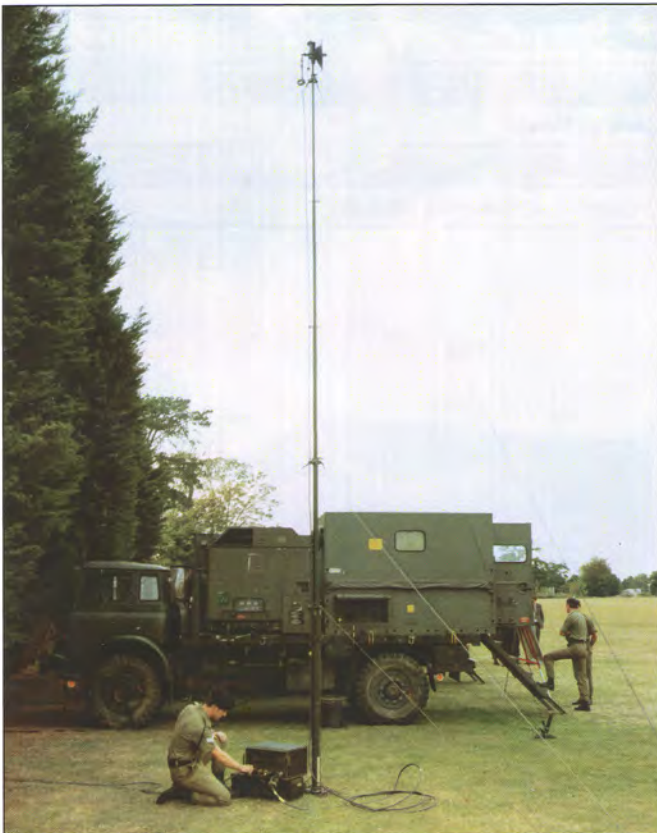
Photo: PU mast field mounted, fully erected and guyed.
